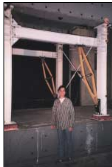
■ A. Natali Sigaher stands in front of the scissor-jack damper system she is testing on the shake table at the University at Buffalo.
