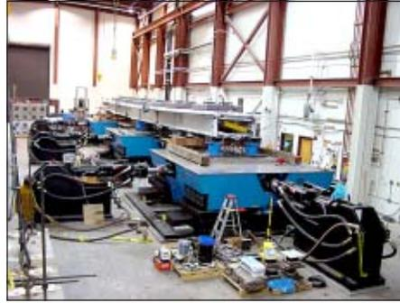
■ A demonstration of the NEESgrid system used this model of a long span bridge supported on two shake tables.
