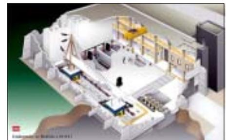
■ *This conceptual drawing shows a cut away view of the dual shake table configuration planned for the UB facility*
