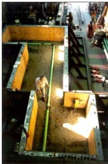
■ *Cornell's facility will allow large scale testing of underground lifelines*
