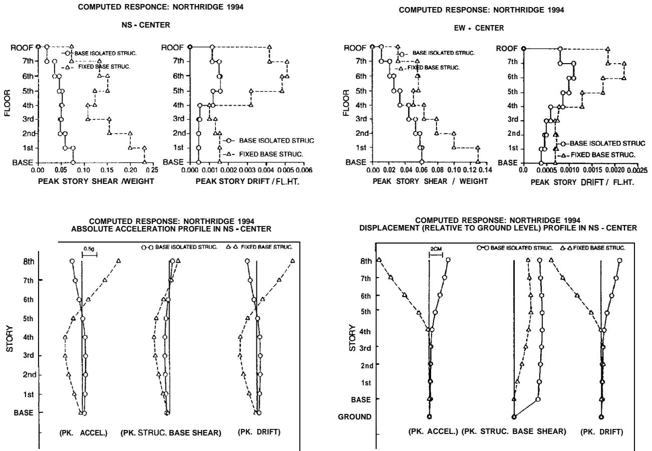
**Figure 4: Comparison Between Base Isolated and Fixed-based Case: (1) Normalized Peak Story Shear and Drift Envelopes in NS and EW Directions; (2) Displacement and Acceleration Profiles at Instants of Occurrence of the Peak Acceleration, Peak Structure Base Shear (above base), and Peak Drift in the NS Direction**
