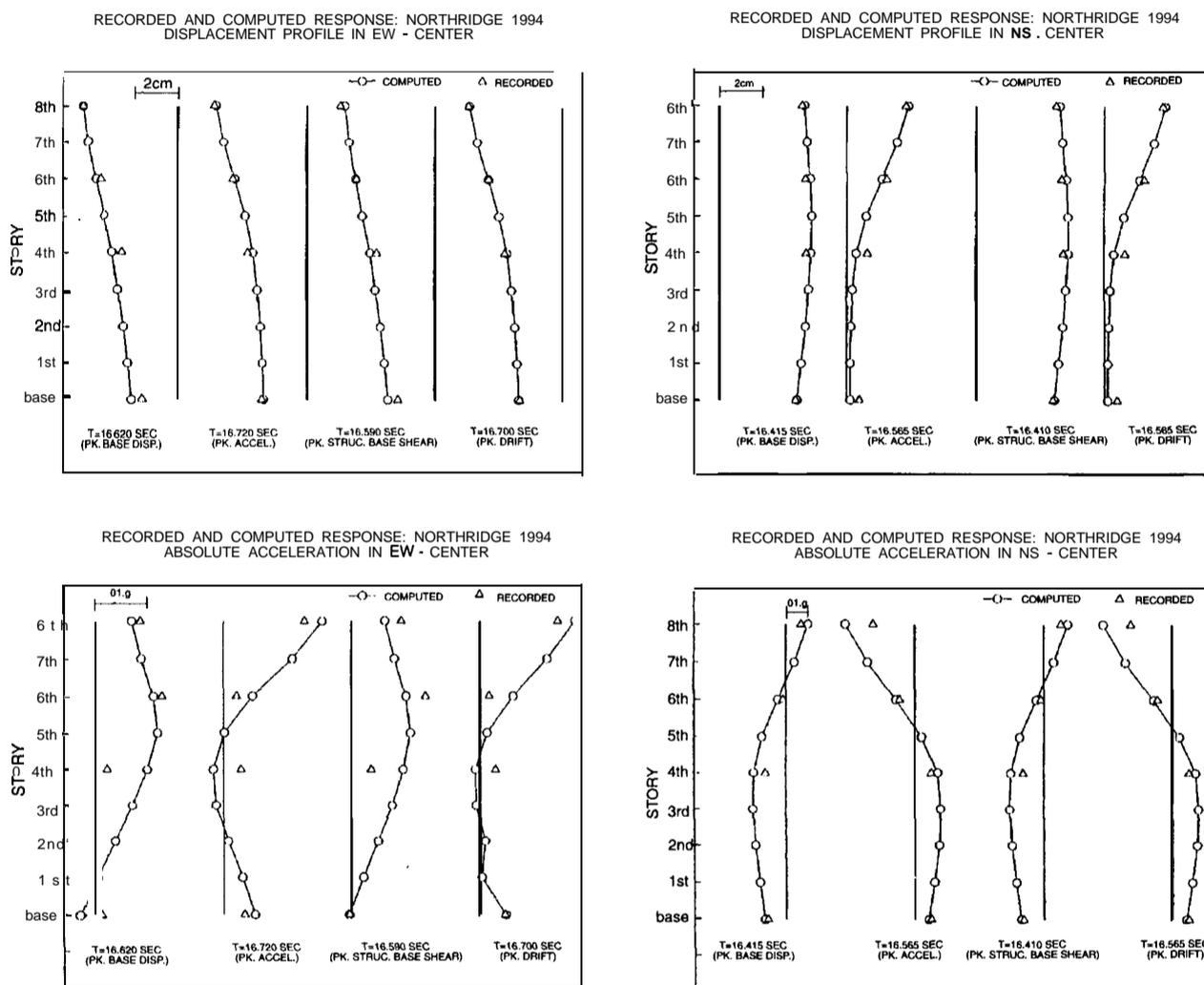
**Figure 3: Recorded and Computed Displacement and Acceleration Profiles at Instants of Occurrence of the Peak Base Displacement, Peak Acceleration, Peak Structure Base Shear (above base), and Peak Drift - in the EW and NS Directions**
