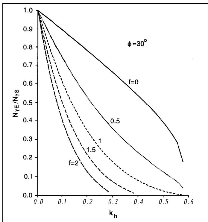
Figure 2. Seismic Bearing Capacity Factor
