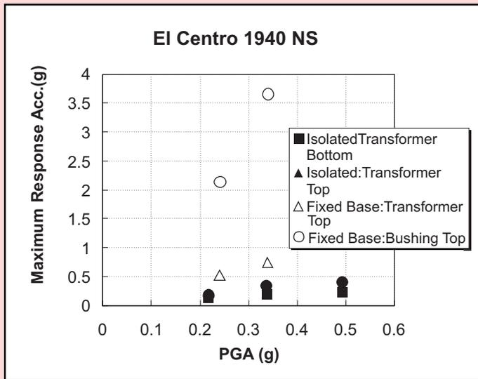
■ Figure 7. Peak Response Accelerations Under Uniaxial Shaking
