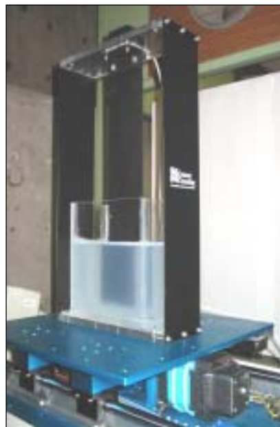
Figure 5. Test setup: A simplified model of a viscous wall
