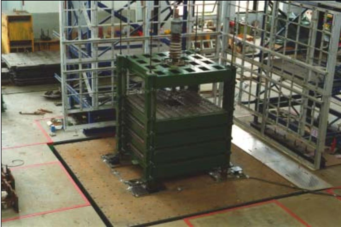
Figure 1. Experimental model of transformer-bushing on shaking table
