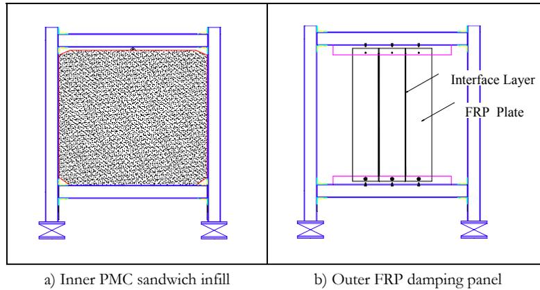
Figure 1. Configuration of a multi-panel PMC infill system
