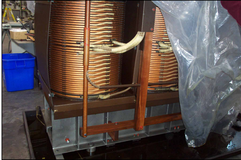
Figure 5. Internal components of a transformer
