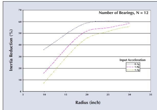
■ Figure 7. Acceleration Reduction by FPS Bearings
