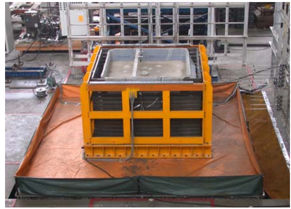
Figure 8. Large-Scale Laminar Bi-axial Shear Box Tests on Shaking Table
