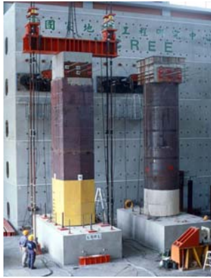
Figure 3. Seismic Retrofit of Full-Scale Bridge Columns
