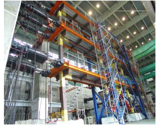
Figure 4. Columns Full-Scale Pseudo-Dynamic Tests of a Buckling Restrained Braced Frame
