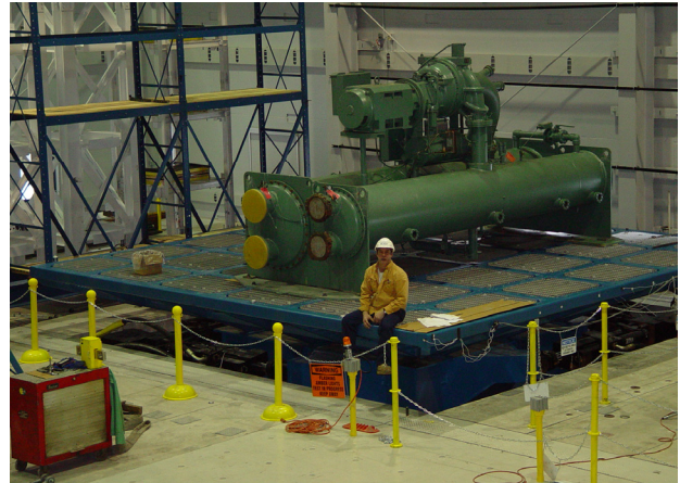
Seismic Fragility Testing of Centrifugal Chiller at MCEER
