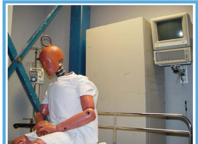
*The inaugural test of the UB Nonstructural Components Simulator (UB-NCS) demonstrated the effects of earthquake floor motions on a full-scale composite hospital room, nonstructural components and contents... including patient.*
